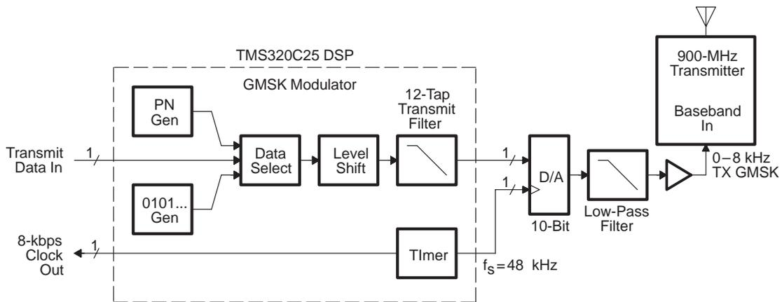
The present GMSK modulator algorithm accepts data from upper OSI layers that has been packetized, error encoded, and scrambled according to Mobitex specifications. In most systems, this is accomplished on a CPU in the application computer or in a separate microcontroller. Ultimately, these functions can occur on the DSP.
