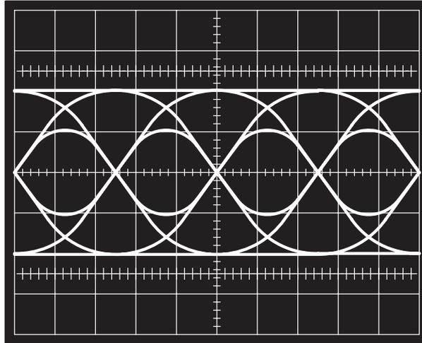
† Signal observed at the output of the transmit filter
